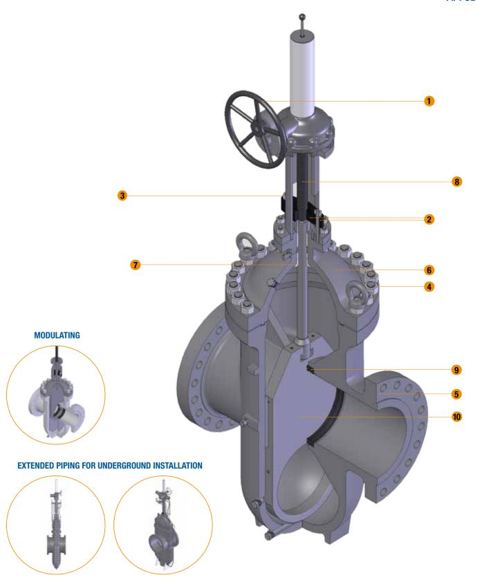
CAST STEEL, CONDUIT TYPE PIPELINE GATE VALVES, SINGLE DISC, NORMAL ACTING OR REVERSE ACTING, OUTSIDE SCREW AND YOKE, RISING STEM, METAL TO METAL OR SOFT INSERT SEATS, REMOVABLE YOKE SLEEVE, GLAND REPACKING UNDER PRESSURE.
