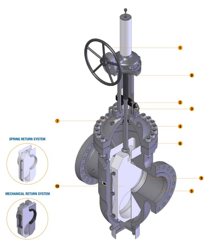
CAST STEEL, CONDUIT TYPE PIPELINE EXPANDING GATE VALVES, OUTSIDE SCREW AND YOKE, RISING SYSTEM, METAL TO METAL OR SOFT SEATS, REMOVABLE YOKE SLEEVE, GLAND REPACKING UNDER PRESSURE.
